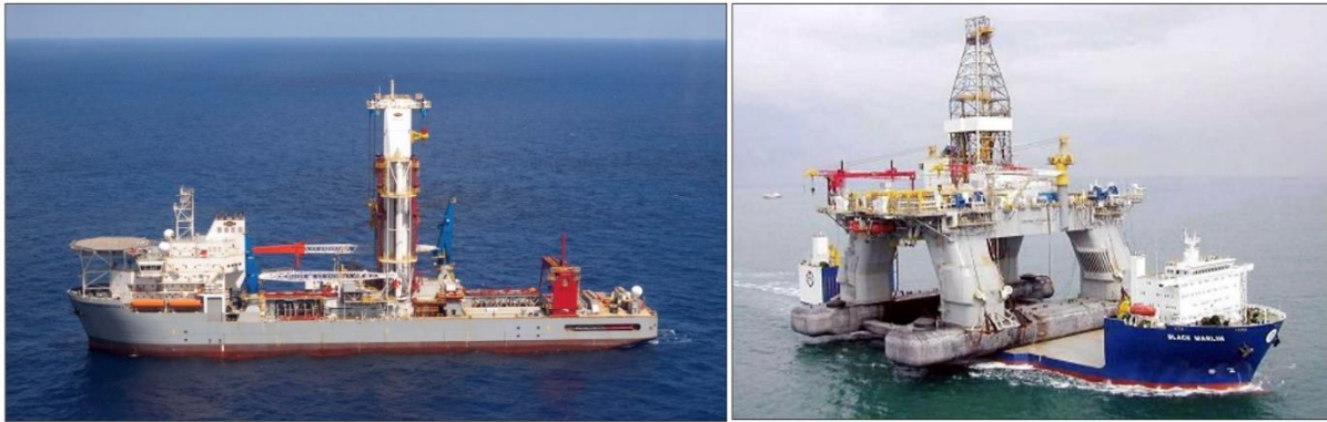
Plate 2: Example of a drill rig, the Noble Globetrotter II (left) and of a semi-submersible, the Deepwater Nautilus, being transported on a heavy-lift ship.
